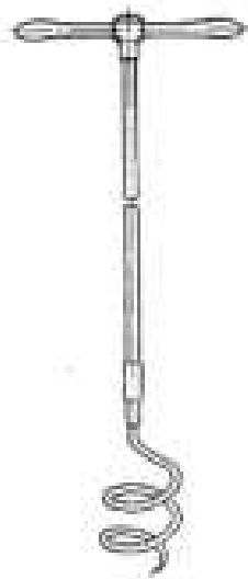
Figure 23.8 : Spiral Auger or Ram's Horn
