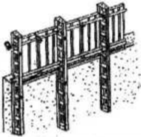
Fig. 5.1A : Single Sided Wall Form (Adjustable)
