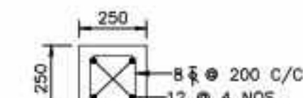
REINFORCEMENT DETAILS FOR COLUMN (SCALE 1:5)
