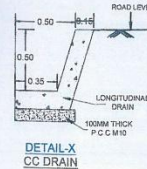
DETAIL-X CC DRAIN
