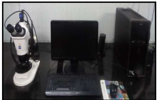
Light microscope used for identification (KL-300LED Carl Zeiss microscope)
