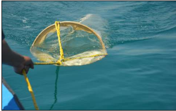
Plankton sample collection by using Bongo net
