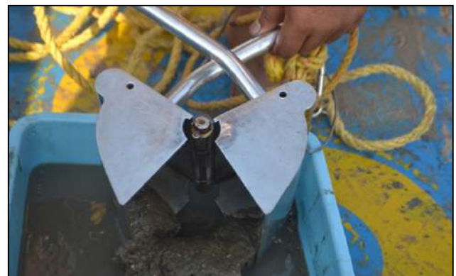
Sediment sample collected by using Van Veen Grab
