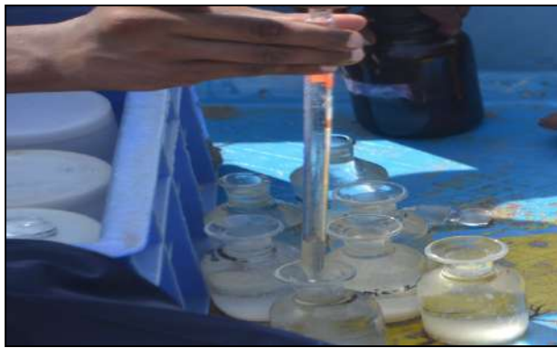
DO estimation by following Winkler's method
