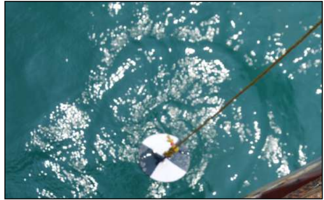
Vertical transparency measurement by using Secchi disc
