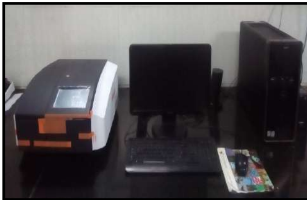
Water analysis using (UV – 1900 UV – VS Spectrophotometry)
