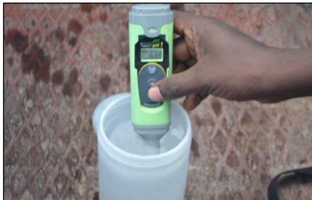
Water pH measurement by using pH pen
