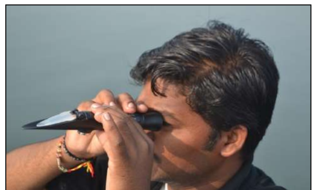
Salinity measurement by using Refractometer
