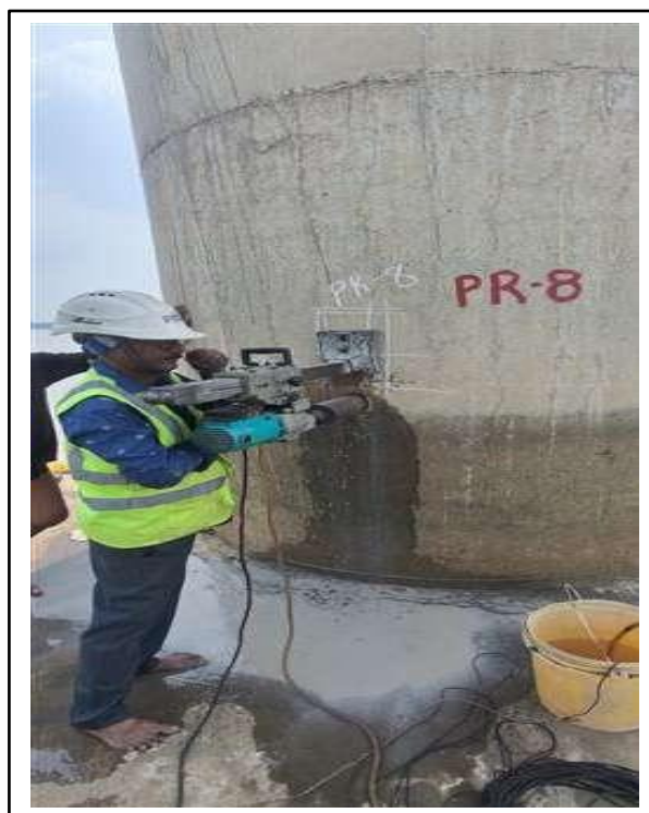
Conducting Core cutting test
