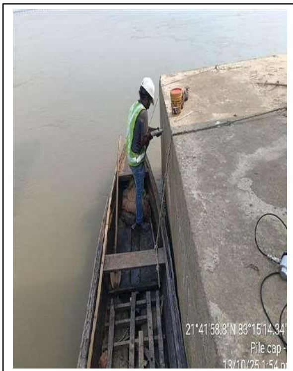
Conducting UPV test
