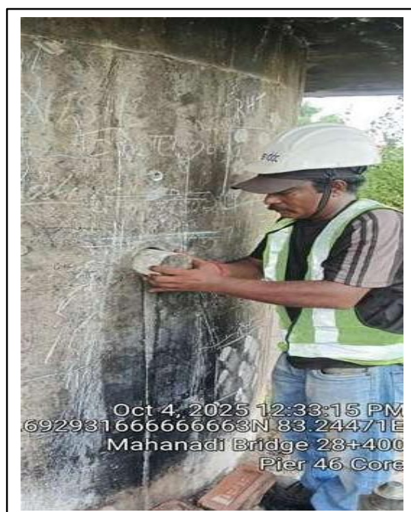
Conducting Core cutting tests
