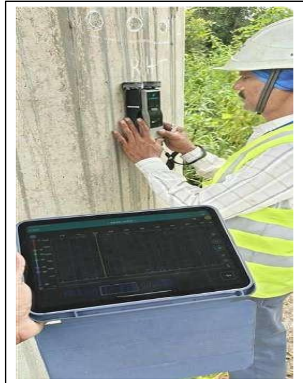
Conducting Concrete cover meter tests
