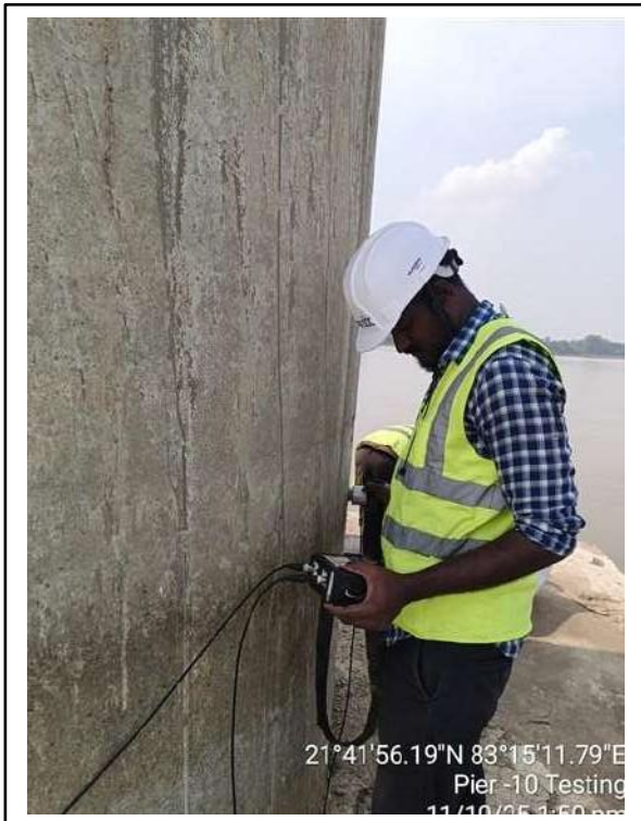
Conducting UPV test
