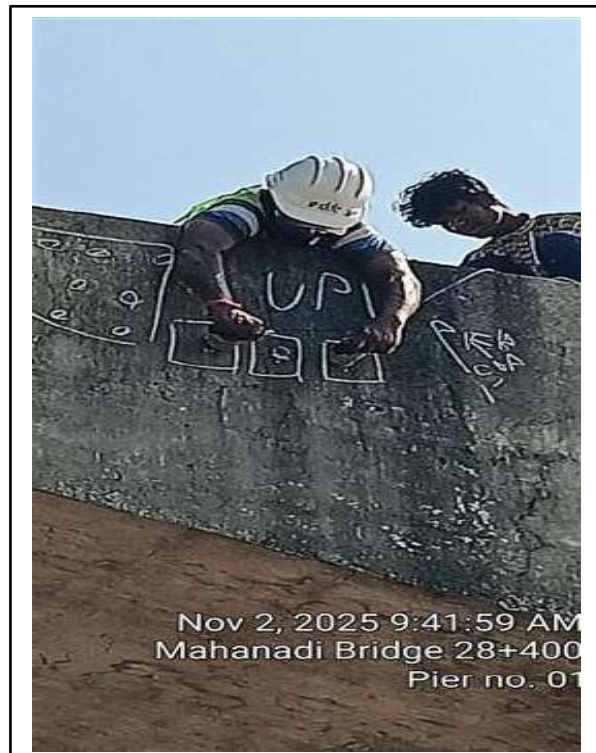
Conducting UPV tests
