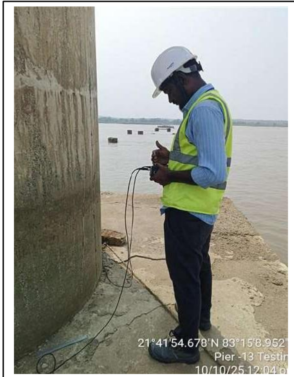
Conducting UPV test
