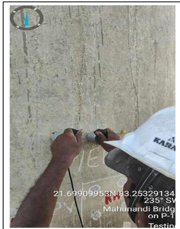
Conducting UPV test
