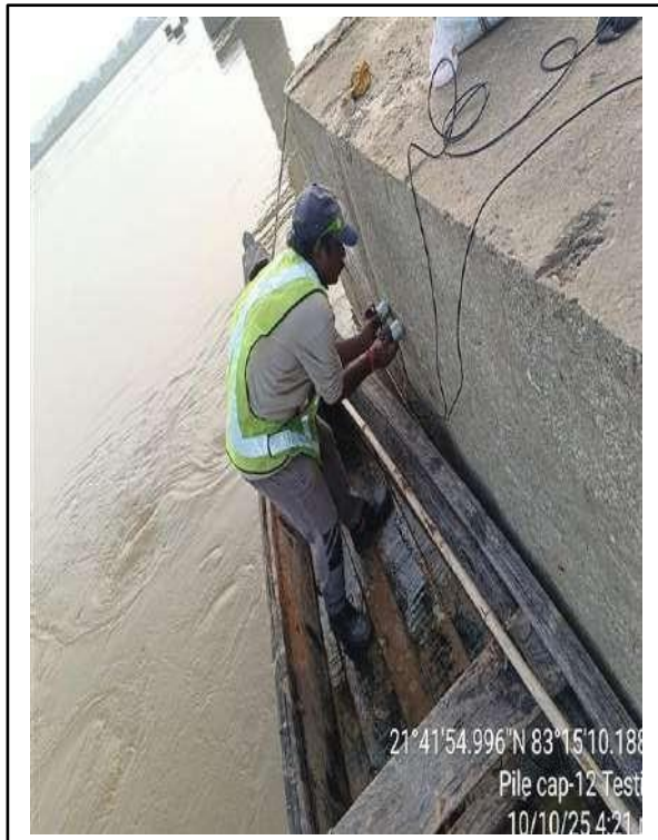
Conducting UPV test
