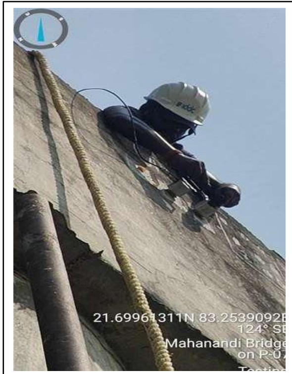
Conducting UPV test
