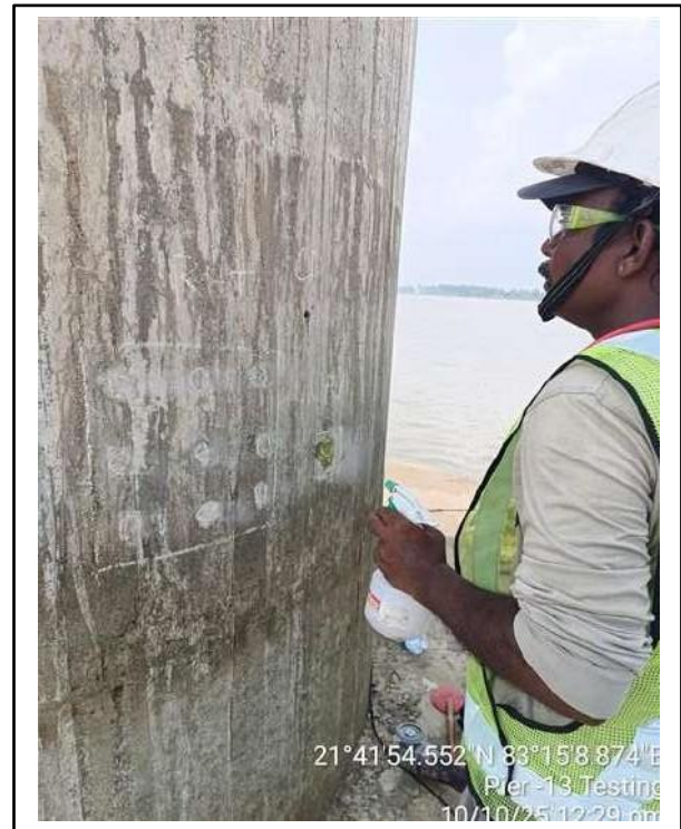
Conducting CD test
