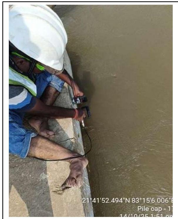
Conducting UPV tests
