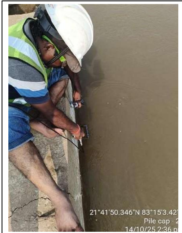
Conducting UPV tests
