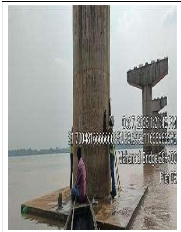
Conducting UPV tests
