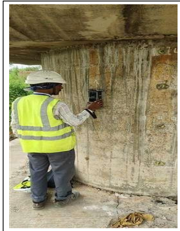
Conducting Concrete cover meter tests
