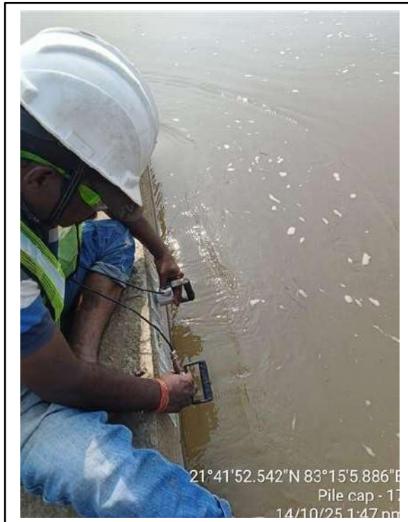
Conducting UPV tests
