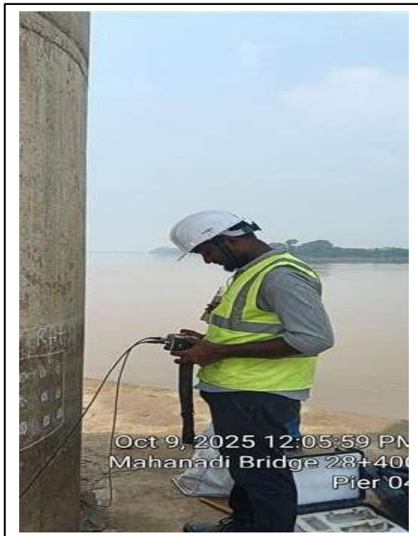
Conducting UPV tests
