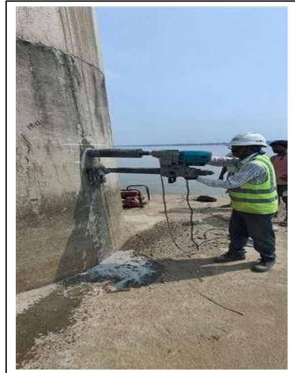
Conducting core cutting test
