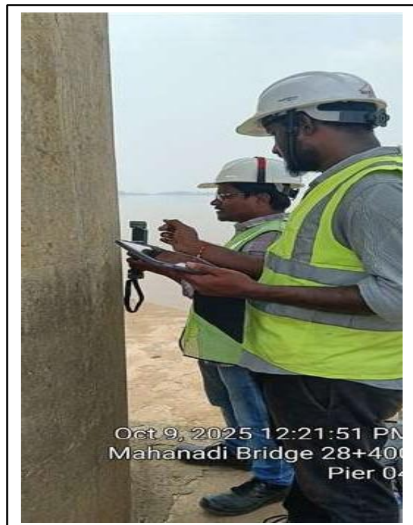
Conducting Concrete cover meter tests
