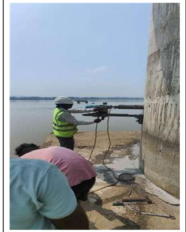
Conducting core cutting test
