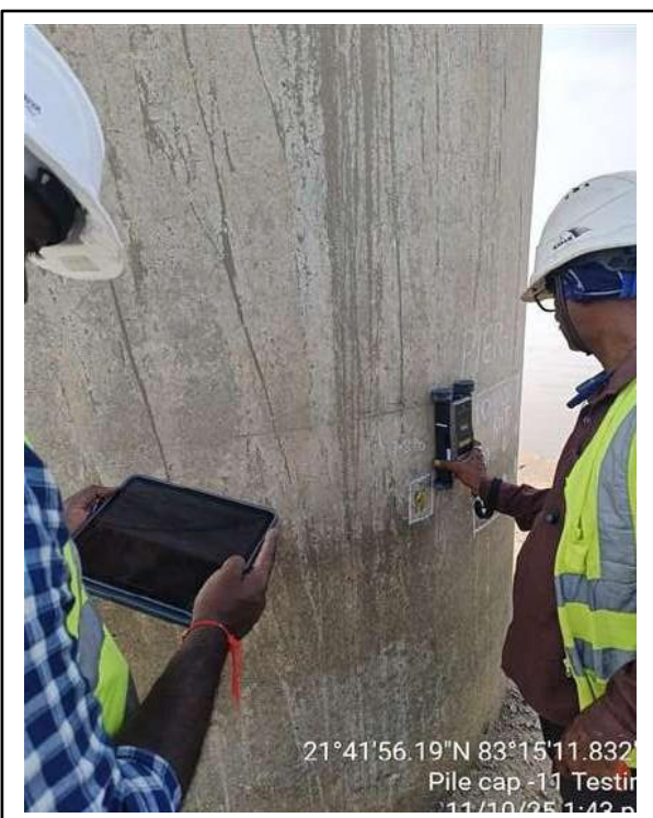
Conducting concrete cover meter test
