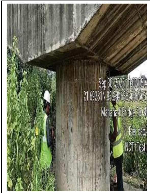
Conducting UPV tests
