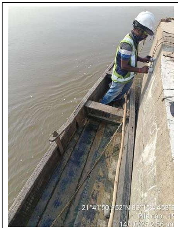
Conducting UPV tests
