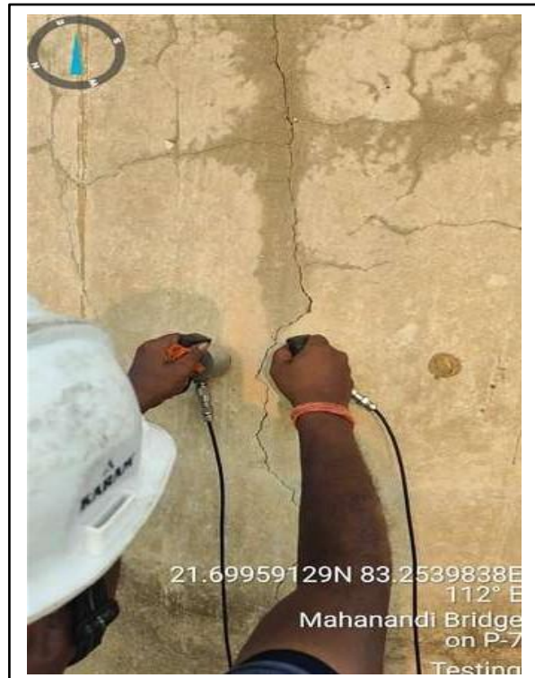
Measuring Crack depth
