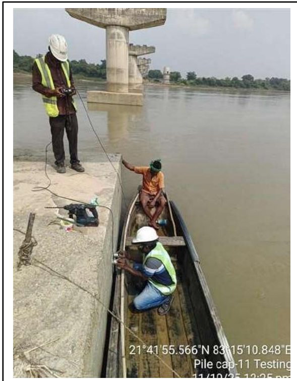
Conducting UPV test
