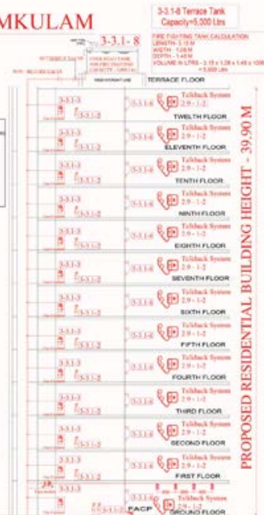
3-3,1-4 WET RISER SYSTEM SCHEMATIC DIAGRAM
